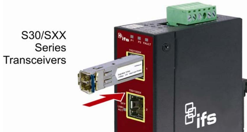
Figure 2-3: Plug in the SFP Transceiver
