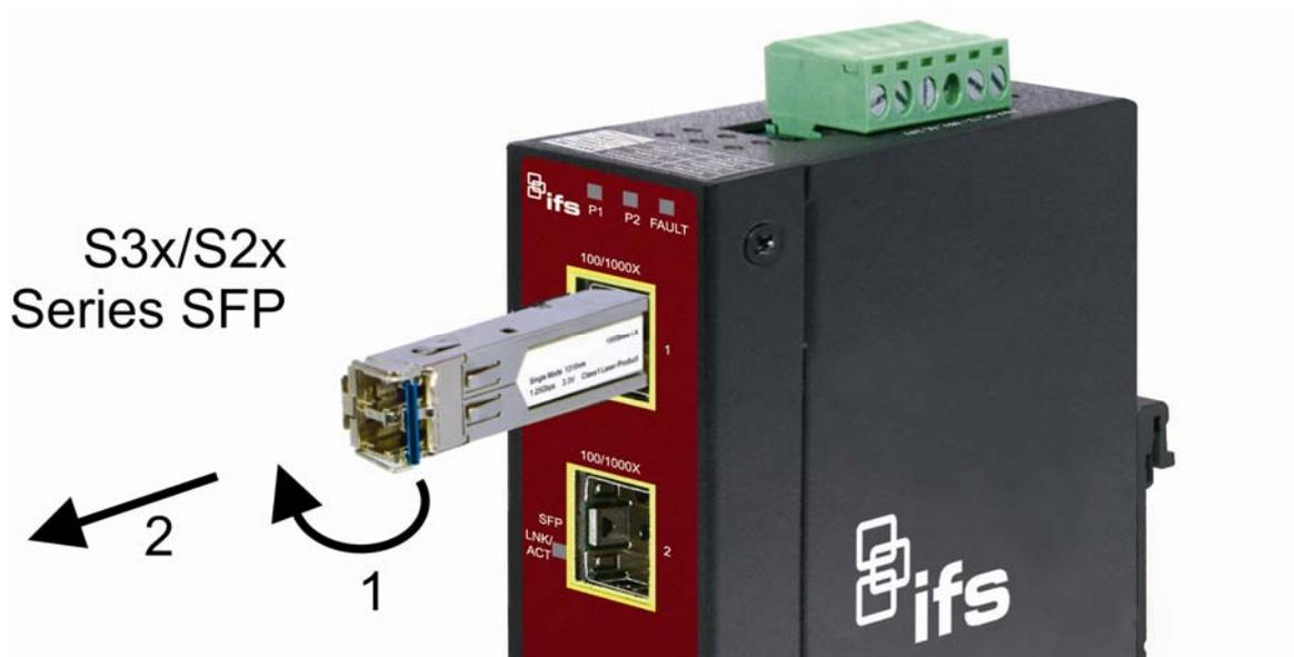
Figure 2-4: Pulling Out from the Transceiver
