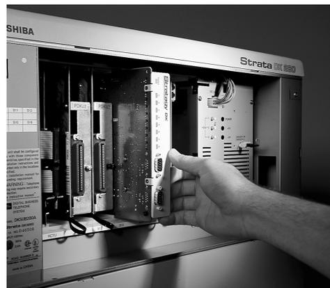
**CAUTION!** Do not hit the board for proper seating. This can damage the Strategy DK components.
