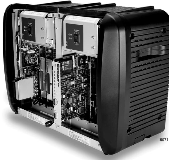
**CAUTION!** Do not hit the board for proper seating. This can damage the Strategy DK components.
