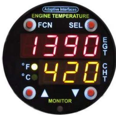
In this mode, Exhaust Gas Temperature and Cylinder Head Temperature are displayed in ENGLISH units. EGT and CHT are displayed in Degrees Fahrenheit.
