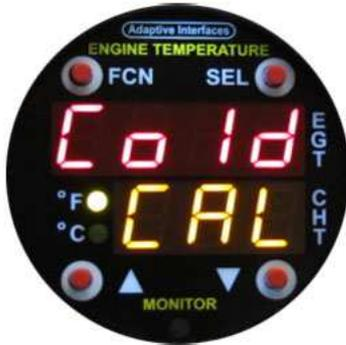
TO PERFORM THIS SETTING, BOTH THERMOCOUPLES NEED TO BE REMOVED FROM THE ENGINE AND PLACED IN AN ICE BATH AT 32° F.
