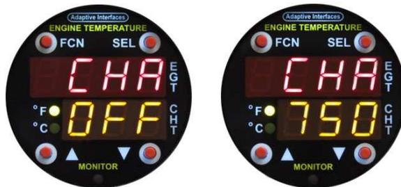
The CHT HIGH TEMPERATURE ALARM can be cycled OFF and from 500 °F to 900 °F in 10 °F steps.
