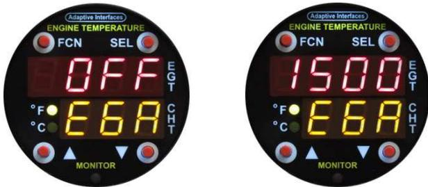
The EGT HIGH TEMPERATURE ALARM can be cycled OFF and from 800 °F to 1900 °F in 10 °F steps.
