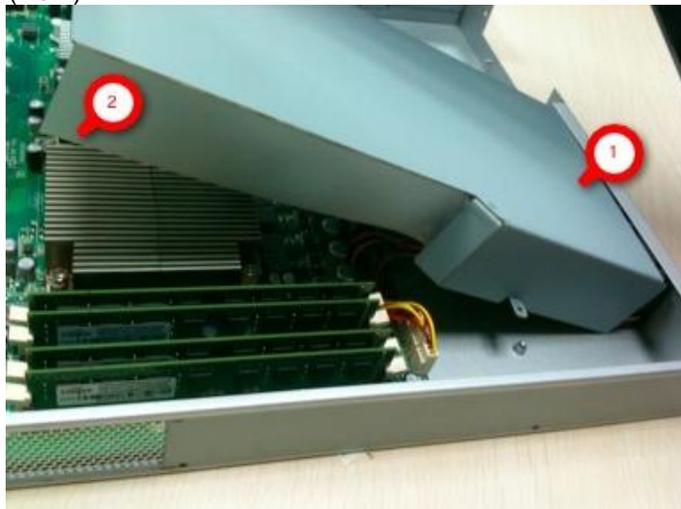
The complete installation of the FAN cover is shown as below.
