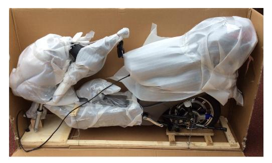
Use the wire cutters to remove the bike from its wooden base. The front forks are attached to a wooden block by the front wheel axle. Undo the axle bolt and withdraw it from the block to release the bike fully from the base. The bike needs to be steadied as you remove the fixings.
