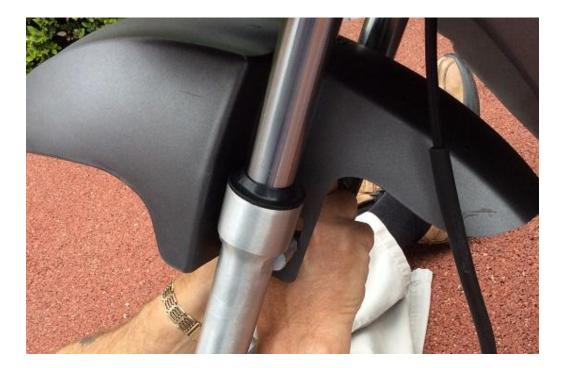
Take the front wheel and ease the brake mechanism into the drum. Line up the wheel centre with the end of the forks. Feed the axle bolt through the fork end and the wheel until you can locate larger aluminium spacer inside the forks. Push the axle through the wheel.
