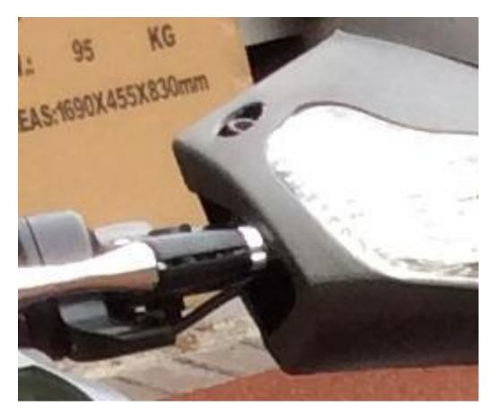
Having pressed the mirror bolts fully home, tighten the securing nut with a spanner. Before fully tightening, adjust the mirror angle to suit your riding position.
