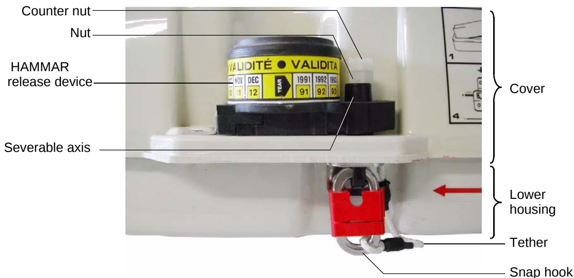
Figure 14: Hammar release device in locked position
