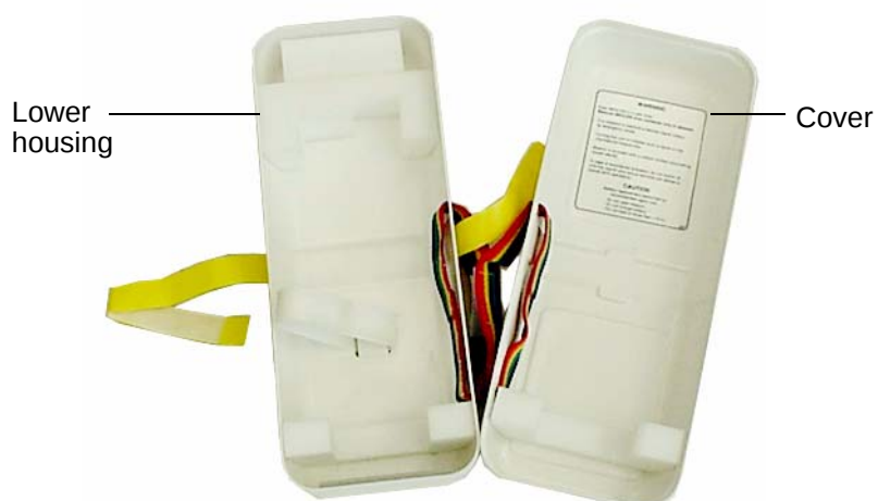
Figure 7: Container for KANNAD 406 S without water switch sensor
