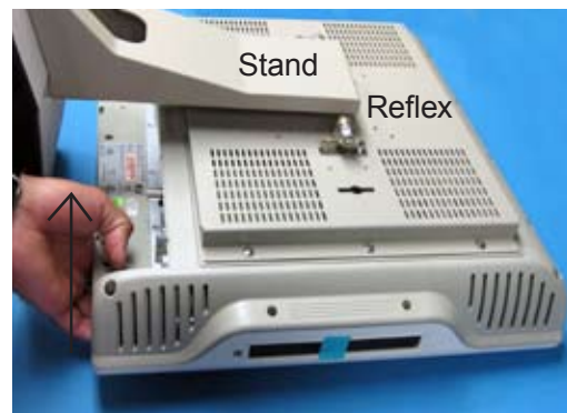
Figure GS-10 Lift Up Bottom Edge
