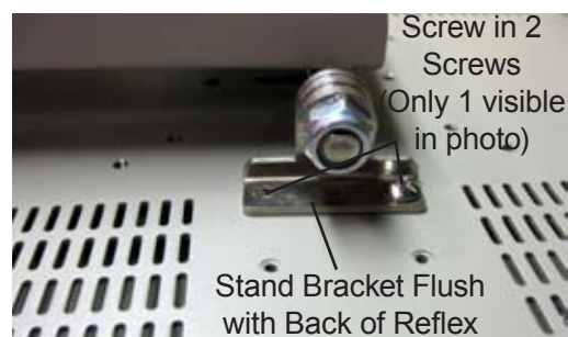
Figure GS-11 Attach Brackets
