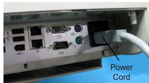
Figure GS-15 Connect Power Cord
