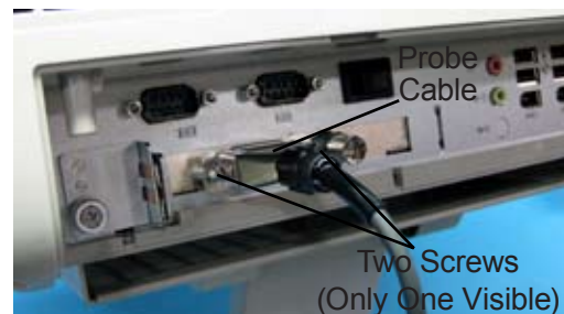
Figure GS-16 Connect Probe Cable
