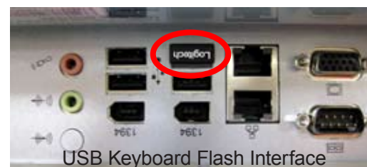
Figure GS-18 Connect USB Keyboard Flash Interface
