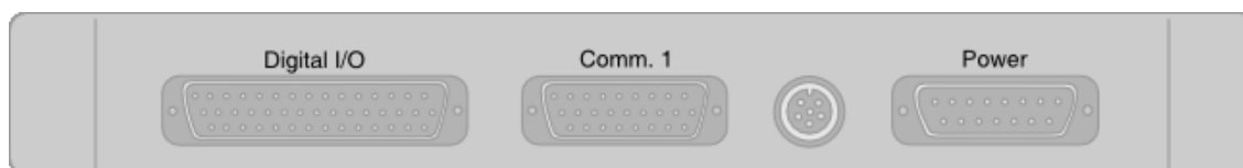
Figure 5-1: Diagram of the connectors on the back panel of an ECPU layer including the 44-pin D-Sub Digital I/O connector and the 9-pin D-Sub Comm port used for serial bus inputs.
