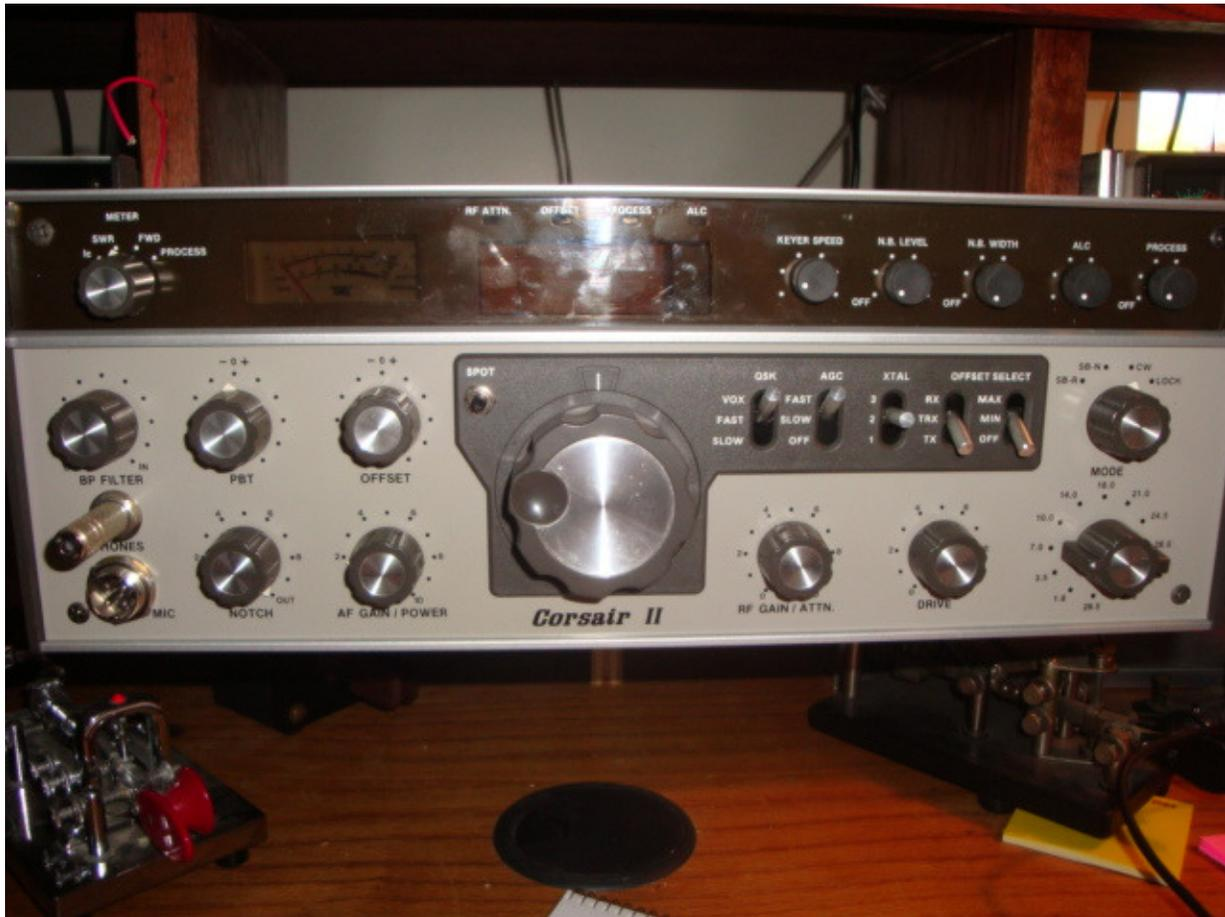
This is my completed Corsair panel. As you can see, the 0-100 logging skirt is now gone from the tuning knob. The DDS operation doesn't suit the use of that anyway. With its capability for "fast" vs. "slow" tuning depending on rate of rotation of the tuning knob, a 0-100 skirt would not be suitable.
