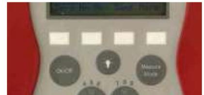
5. After the MFT is on, and before any connections are made to the PIT5000, press the ZERO soft key (white, rectangular key on left hand side below display) to zero the pressure module.
