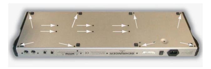
Fig. 3.1: Removing the bottom panel
