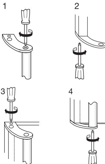
2. Fit the top handle bracket on the top left-hand side of the door (3) and screw the handle rod to the bottom handle bracket (4).
