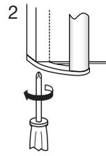
10. Unscrew the top handle bracket from the door (3) and screw onto the bottom right-hand side of the door (4).
