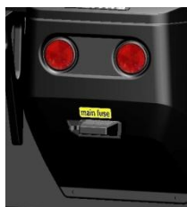
position of the main fuse
