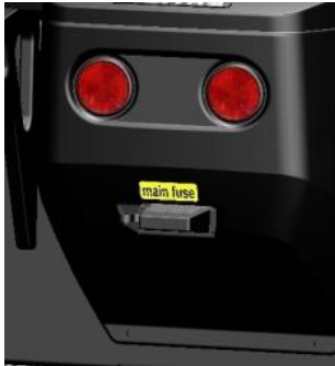
place of the main fuse
