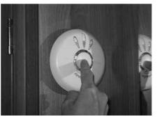
The unit will emit a loud (85dB at 3 meters) alarm for around 5 seconds and stop automatically.
