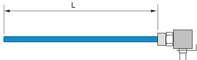
Length L in mm is calculated with the formula:  $(Nt - Nc) * 55 - 16$
