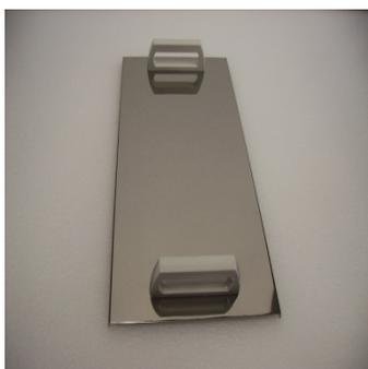
When the instrument is not in operation, the reagent troughs should be covered with the two stainless steel covers supplied to minimize the evaporation of the solvents.
