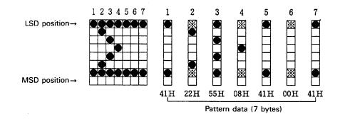
As the model utilizes the half-dot printing method, it is not capable of positioning successive dots in the printing direction (between print). Therefore, pattern specification in the position "\*" to the right of the position " $\bullet$ " in the diagram above will not be registered as pattern data.
