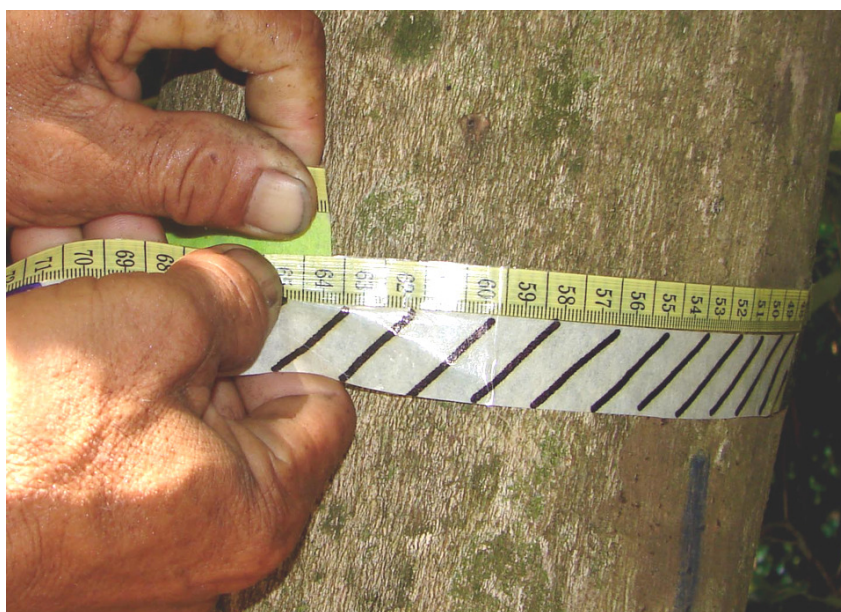
Figure 2: Adjusted measure tape with scales for girth and colour diameter classes
