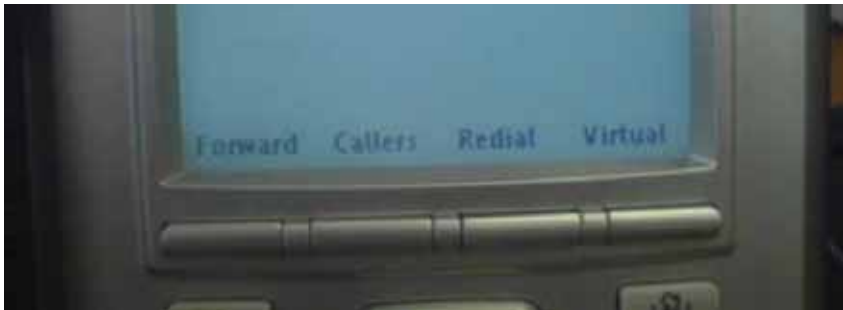
Figure 6: Virtual soft key — Avaya 1220 IP Deskphone
