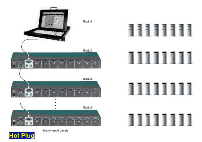
The KVM Switch supports "Hot Plug" function for easy addition or removal of PCs. The user can arrange or maintain PCs as follows:
