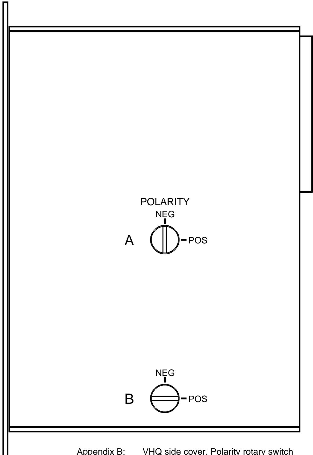
Appendix B: VHQ side cover, Polarity rotary switch
