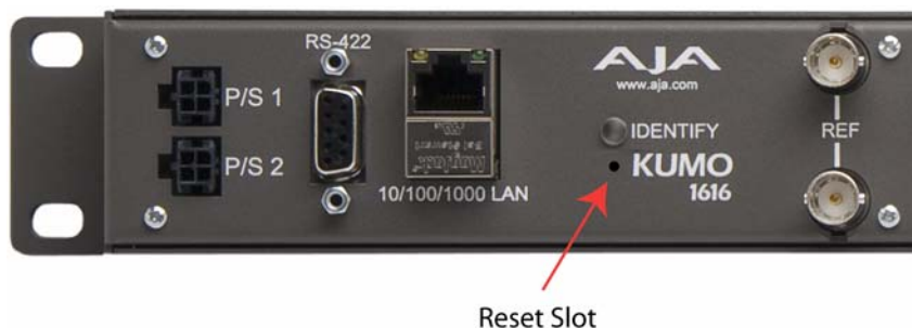
KUMO Rear Panel and Reset Slot
