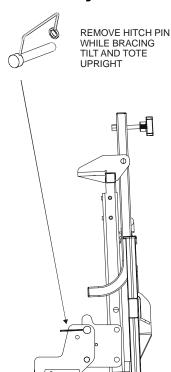
ONCE PIN IS REMOVED, THE TILT AND TOTE CAN BE LOWERED JUST BELOW PARALELL WITH THE GROUND BEFORE RESTING ON ITS MECHANICAL STOPS.
