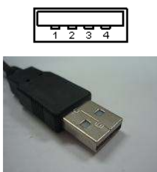
Figure 3: Type A USB connector.
