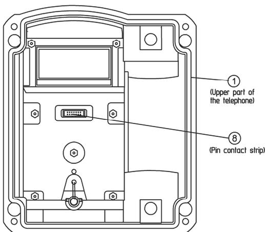
**Figure 7: Inside View of Telephone upper Part**
