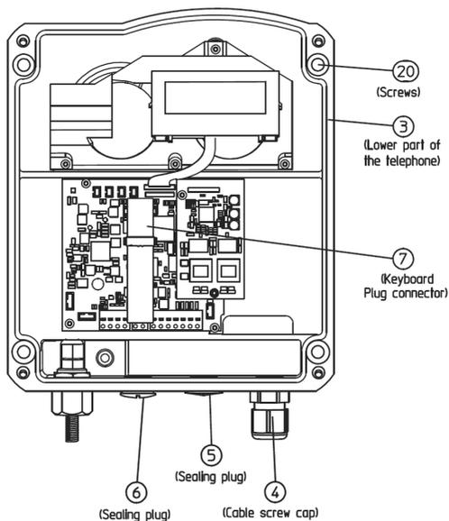
**Figure 8: Inside View of Telephone lower Part**
