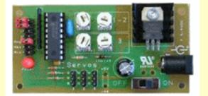
Board Size: 3-4/8" L x 1-3/4" W x 1/2" H Board is pre-assembled and tested.
