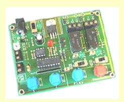
Board Size: 4" L x 3" W x 1/2"H Mechanical relay rated 30V @ 2Amps
