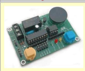
Board Size: 2-3/4" L x 1-1/3" W Controller has 7-bit Resolution. Power Requirements: 5Vdc @ 1 Amp Assembled and Tested
