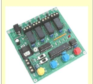
Controller is pre-assembled and tested. Controller has 7-bit Resolution. Board Size: 4" L x 4" W x 1/2" H The Wizard- 4 Controller Board or Programmable 4 - Channel Relay module will record and playback up to **25 minutes** of controlled ON and OFF action for 1 - 4 Outputs Relays.
