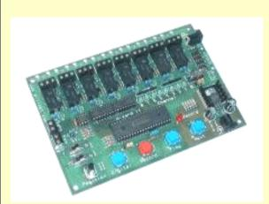
Board Size: 6-5/8" L x 4-1/2" W Wizard - 2 Board is pre-assembled and tested. Controller has 7-bit Resolution.
