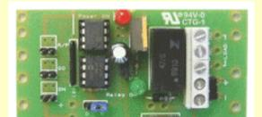
Controller is pre-assembled and tested. Board Size 3" L x 1-1/2" W x 9/8" H
