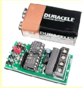
Controller is pre-assembled and tested. Board Size: 1-7/8" L x 1" W x 5/8" H
