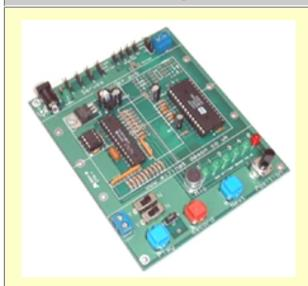
Board Size: 5" L x 4-3/16" W Power: 9 Volt dc @ 2 Amp. Controller has 7-bit Resolution.
