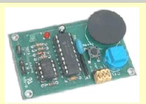
Board Size: 2-3/4" L x 1-1/3" W Controller has 7-bit Resolution. Power Requirements: 5 Volt dc @1 Amp Controller is pre-assembled and tested.
