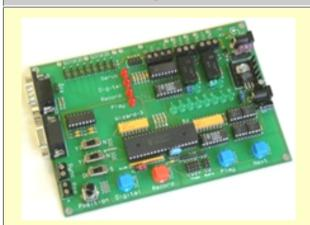
Board Size: 6-5/8" L x 4-1/2" W Wizard - 3 Board is pre-assembled and tested. Controller has 7-bit Resolution.
