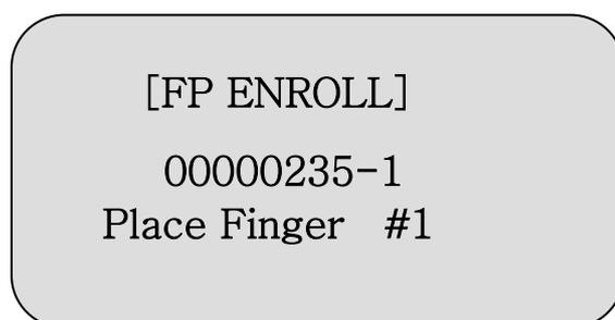
On the screen 00000235-1 means that user's fingerprint will be enrolled the first fingerprint on the ID 235.
