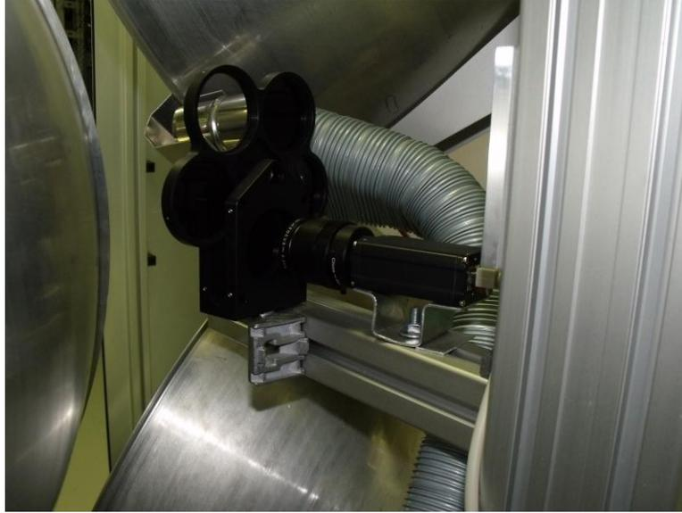
Figure 2-20. The CCD camera and filter wheel. Photo courtesy of Ben Erickson.
