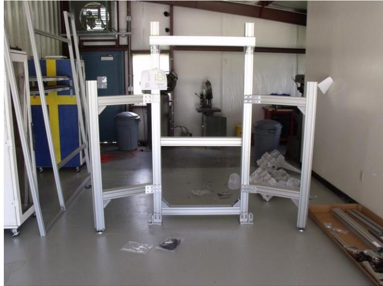
Figure 2-1. The frame of the simulator at the beginning of construction. Photo courtesy of Ben Erickson.
