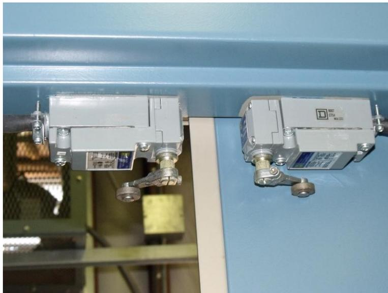
Figure 2-14. Two safety interlocks protecting the rear doors during operation of the simulator. Photos courtesy of Ben Erickson.
