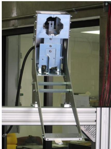
Figure 2-8. Each mirror has a holder assembly (shown above) which allows for coarse and fine adjustment of the focal point. Photo courtesy of Ben Erickson.
