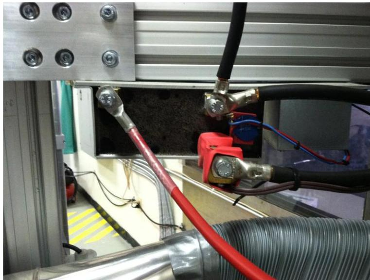
Figure 2-6. Ignition unit mounted below its corresponding mirror/lamp assembly. Photo courtesy of Ben Erickson.
