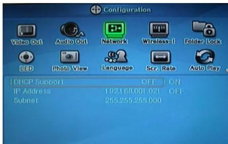
4. Move to 'IP address', 'Subnet' and press "OK". The input box will be displayed and you can enter the number with the "Direction" or "Number" button. Finally, press "ENTER" for saving configurations.
