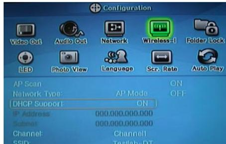
**When connecting Ad-Hoc Mode, manual settings of IP address and Subnet mask will be needed.**
