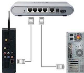
Connect LAN cable to LAN port between IP Router or Hub. In this case, you have to use Direct LAN Cable type generally.
