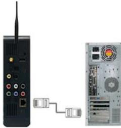
Connect LAN cable to LAN port between Freecom MediaPlayer and PC. In this case, you have to use a Cross-wired LAN cable.
