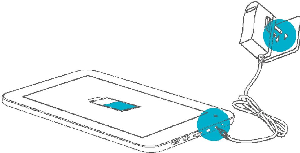
Please make sure that the battery is fully charged before your first use. To charge the battery, please connect the matching charger to a power outlet and insert the DC jack end into the charge interface of LQ8. After a few seconds, the eXiom logo appears on the screen followed by a picture of a battery being charged. After a few seconds the screen will go blank. While the battery is charging, you can view the charging progress by pressing the power button.
