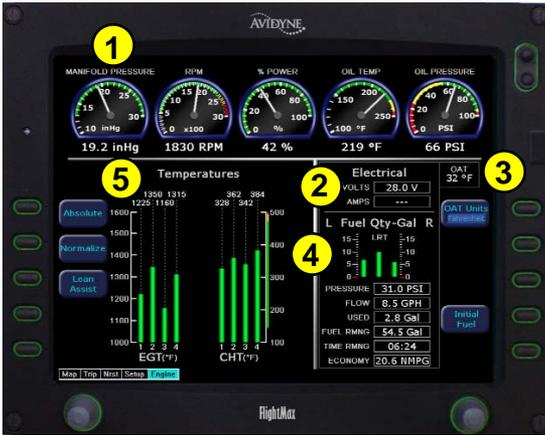
The Engine page is divided into four main sections plus an OAT gauge:
