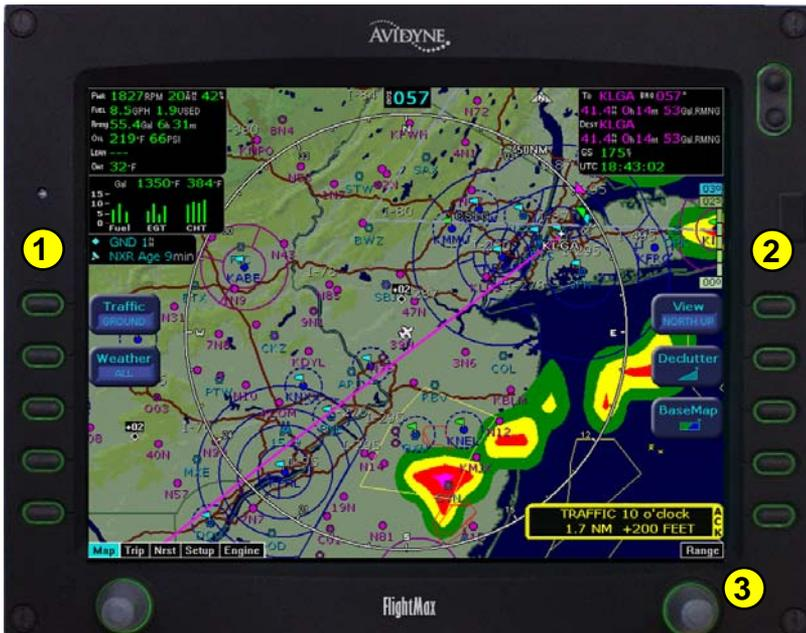
1. **Sensor Functions** - Control overlay and modes of available sensors. Buttons are only displayed for those sensors that are installed in the aircraft.
