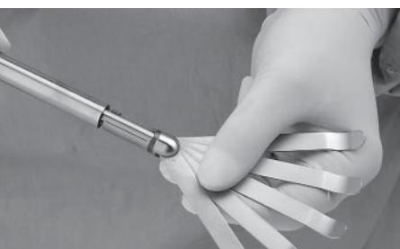
Unscrew the sheath tube and remove it from the internal part with the fan by turning counterclockwise.
