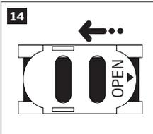
7. Insert all 4 batteries and wait until the LED indicator starts blinking indicating successful micro-controller operation. The system is now running in Wake-Up mode for 3 minutes to configure the system by SMS text messages (see **5. CONFIGURATION METHODS**).
