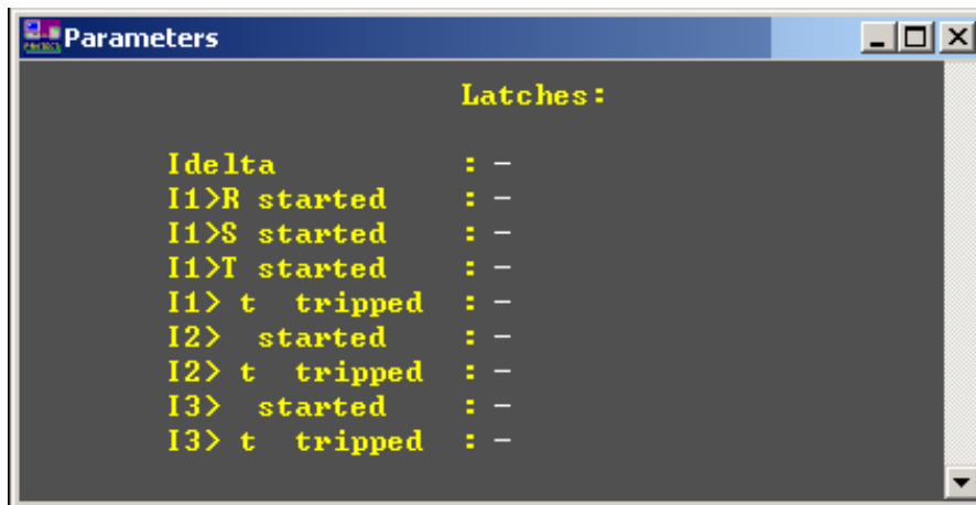
Fig. 11 Latching the status signals of the overcurrent function, three voltage levels (Protect for Windows).
