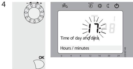
The display shows the hours flashing .
