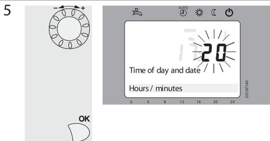
The display shows the minutes flashing.
