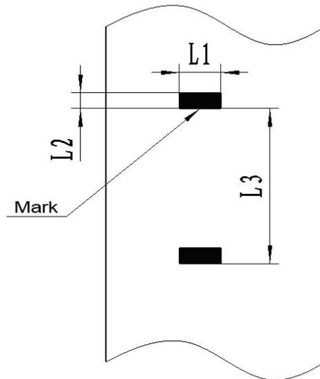
Figure 2.2-1 Schematic diagram of mark position
