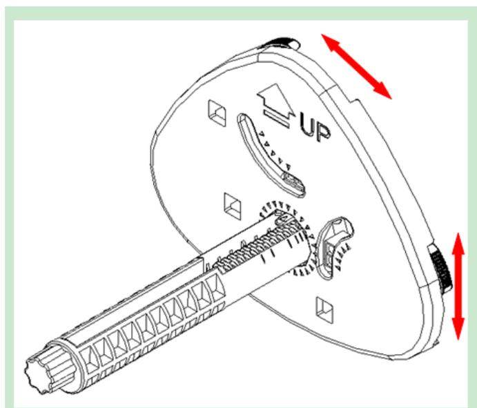
Figure appendix 3.1-15 Adjusting paper near end sensor on cantilever paper holder
