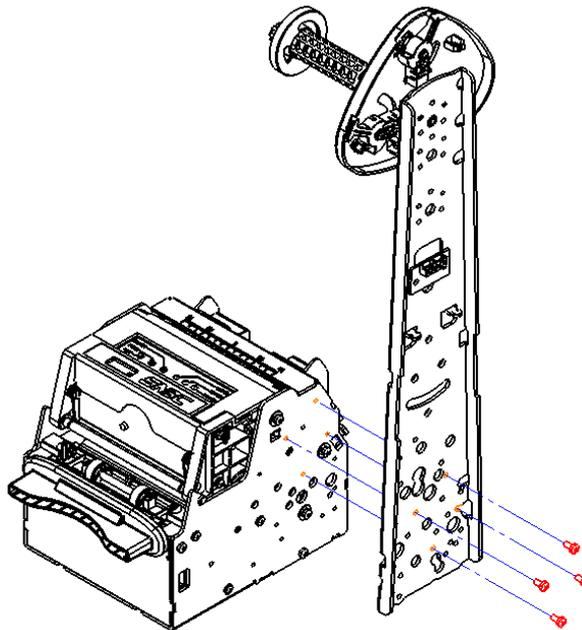
Figure appendix 3.1-6 Cantilever paper holder installed on the right (90°)
