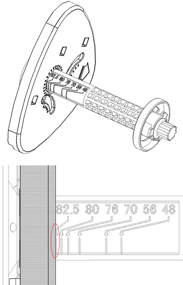
Figure appendix 3.1-14 Scale marks on paper roll shaft of cantilever paper holder
