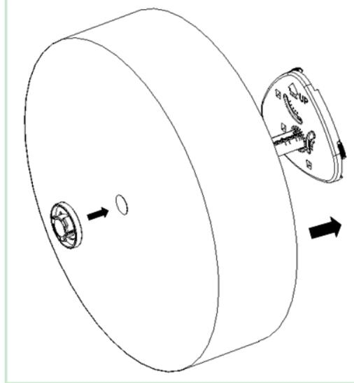
Figure appendix 3.1-16 Replacing paper roll
