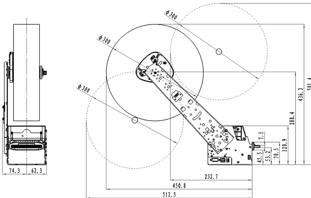
Figure appendix 3.1-11 Installing cantilever paper holder at left side
