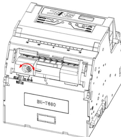
Figure 4.2-2 Adjust the paper guide fixing screws
