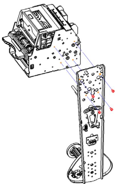
Figure appendix 3.1-2 Cantilever paper holder installed on the right (-90°)
