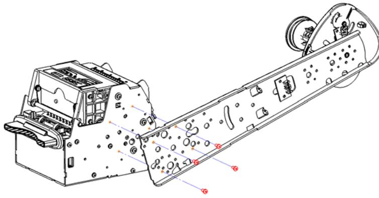
Figure appendix 3.1-4 Cantilever paper holder installed on the right (15°)
