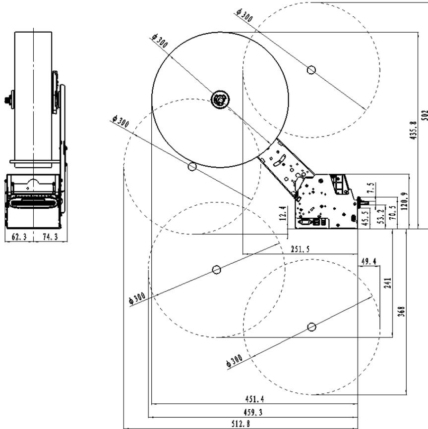
Figure appendix 3.1-10 Installing cantilever paper holder at right side
