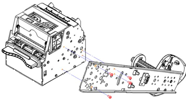
Figure appendix 3.1-3 Cantilever paper holder installed on the right (-45°)
