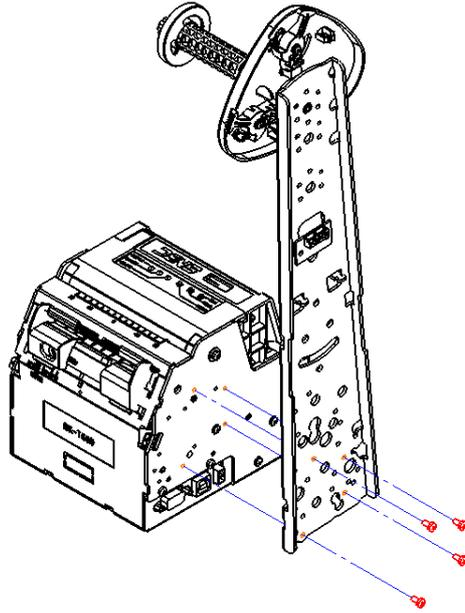
Figure appendix 3.1-7 Cantilever paper holder installed on the left (90°)
