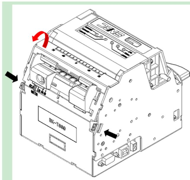
Figure 5.1-1 Cleaning mark sensor
