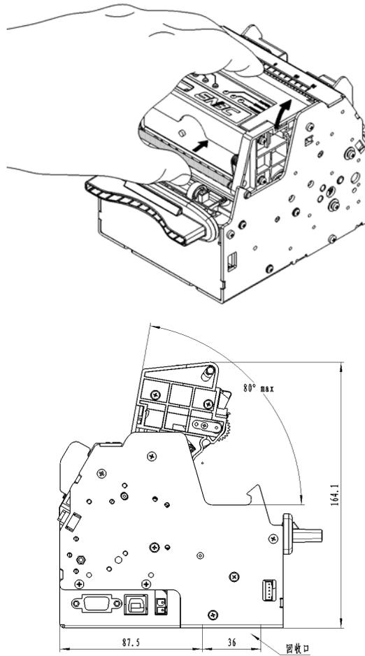
Figure 4.8-2 Printer space with standard paper holder
