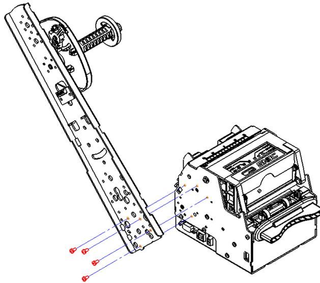
Figure appendix 3.1-8 Cantilever paper holder installed on the left (60°)
