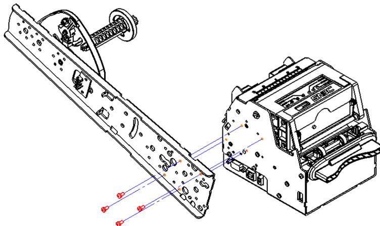
Figure appendix 3.1-9 Cantilever paper holder installed on the left (15°)
