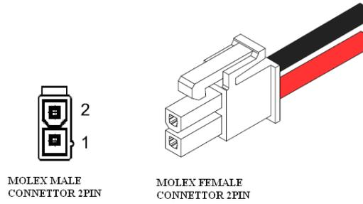
**Figure 6.5-1 Power socket and connector**
