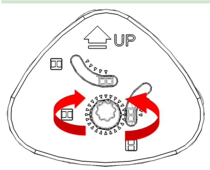
**Figure appendix 3.1-12 Installing cantilever paper holder at left side**
