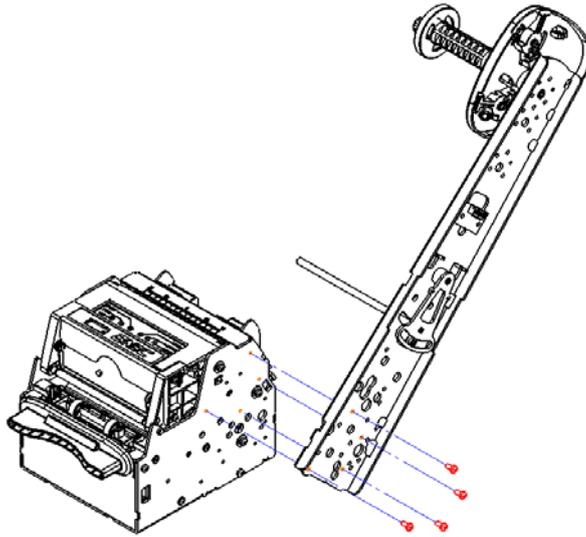
Figure appendix 3.1-5 Cantilever paper holder installed on the right (60°)
