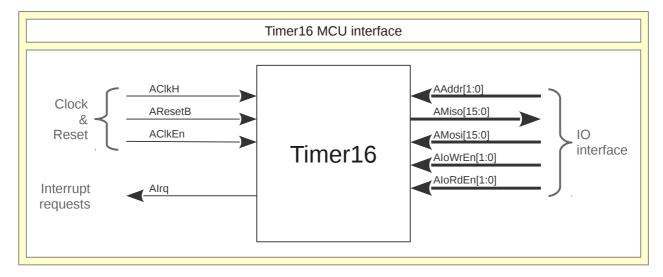
When enabled, timer starts counting from zero up. There are 2 configurable compare values: CmpA and CmpB. When timer counter reaches one of these values it indicates this event by a flag accessible to the software. It can generate IRQ if IRQ source is enabled (see table below). It can optionally restart from zero, stop or copy CmpB to CmpA. These functions can be enabled by the corresponding bit in the control register (see table below).
