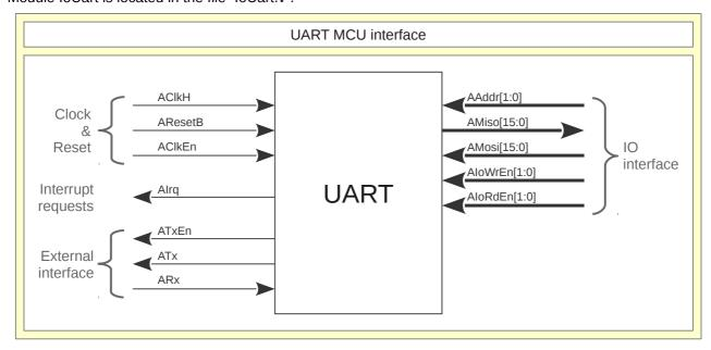
UART transmits and receives data using RS232 interface. It has internal 4-byte buffer for transmission and 4-byte buffer for reception. Signal ATxEn is used to enable or disable transmission output. Implementation on
