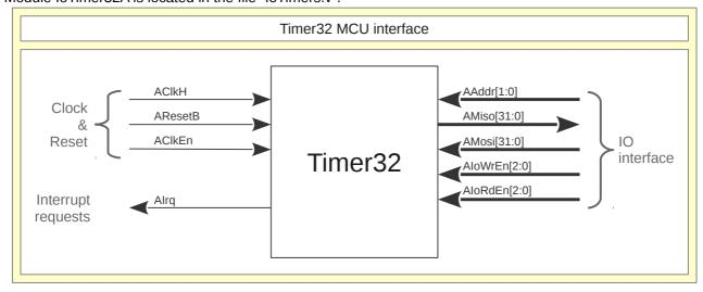
32-bit timer is very similar to a 16-bit one described before. The main difference is the counter width.
