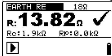
Figure 5.38: Resistance to earth, measurement of a lighting protection system
