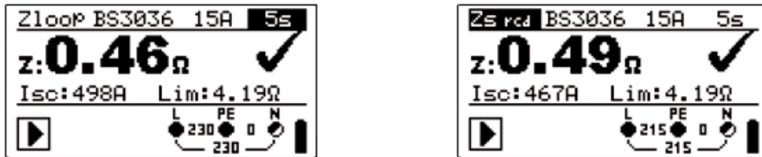
Figure 5.29: Examples of loop impedance measurement result
