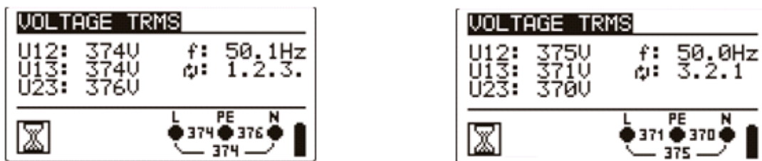
Figure 5.7: Examples of voltage measurement in three-phase system
