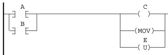
In the above example, either A *or* B provides a true logic path to all three output instructions.
