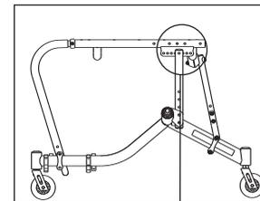
**H. REAR AXLE ASSEMBLY****1. Center of Gravity Adjustment**
