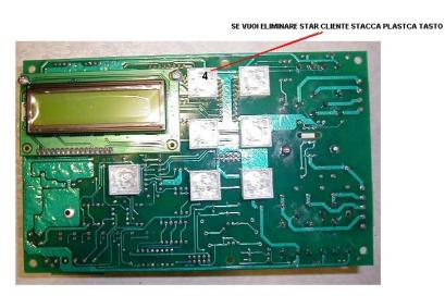
Remove the plastic button to disable START from the control panel
