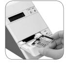
Immediately place the cassette into the analyzer drawer with the black reaction bar toward the analyzer and the brown magnetic stripe on the right.
