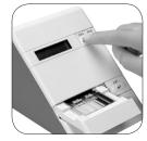
Press the **DATA** button on the analyzer once or twice (depending on the test cassette) to view remaining results.
