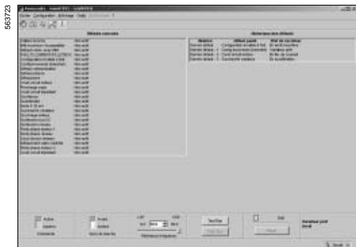
Fault management with PowerSuite for PC
