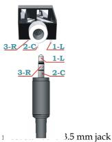
This is 3.5 mm Audio jack female connector and work with headphones. Note the signal is Mono i.e. Left and Right channel info is same.
