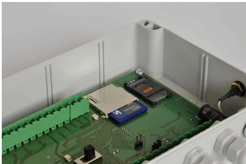
Fig 5. After SIM card installation
