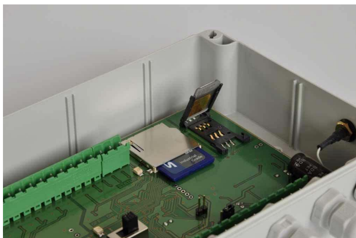
Fig 4. Observe correct orientation and insert SIM card
