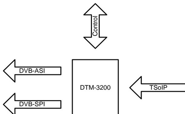
Figure 2. The DTM-3200 configured as IP-to-ASI converter
