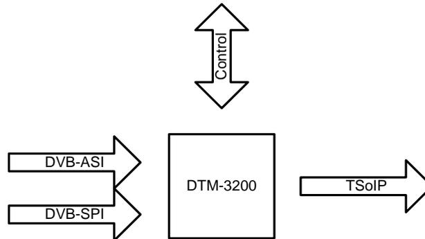
Figure 3. The DTM-3200 configured as ASI-to-IP converter
