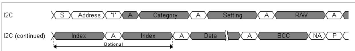
Figure 7. Command (upper sequence) and response (lower) sequence for I<sup>2</sup>C
