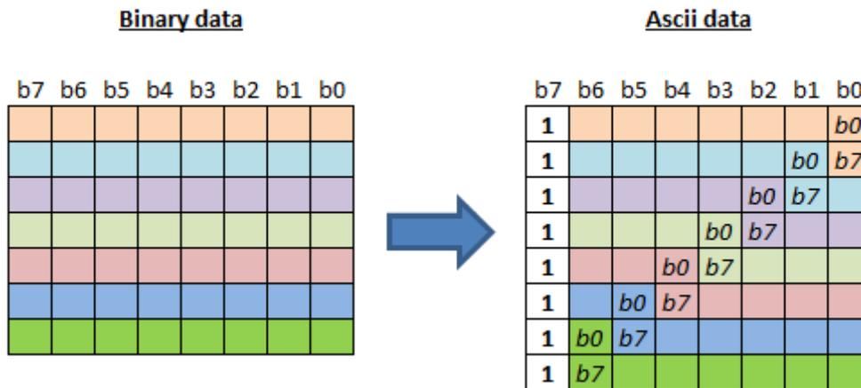
Figure 8. ASCII encoding for firmware update data
