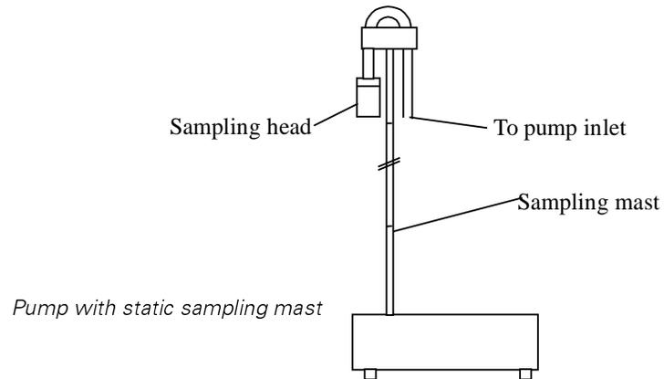
Note :- The sampler should never be run without a filter on the inlet.
