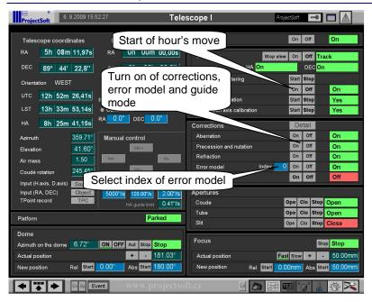
Turn on corrections (aberration, precession and nutation, refraction and error model) and selecting index of error model is possible only when is stop hour's move.
