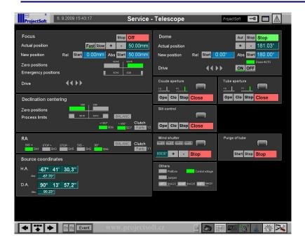
On service screen are visible all system of telescope with end position sensors. When any problem with telescope is possible find out problem on this screen.
