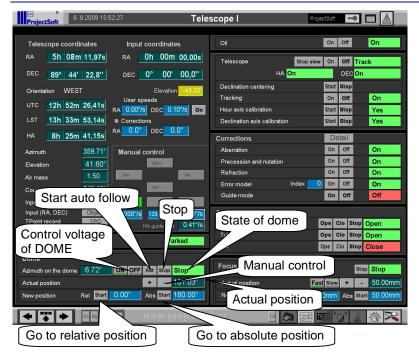
For controlled of dome you must turn on control voltage for dome, when you click on button "ON" in section "Dome". **Attention** – tension is on trolley wire.
