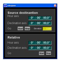
After set RA and DEC coordinates, click on start button and telescope automatically slew on set point position. Condition for slew:
