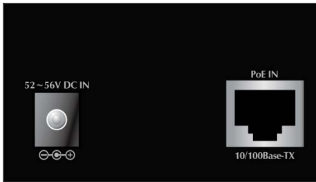
Figure 2-3: MC252-1T-1CXP rear panel
