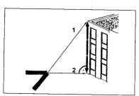
Indirect Measurement - determining a distance using 3 measurements
