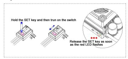
Note4: If you don't release the "SET" key after the red LED begins to flash, the ESC will enter the program mode, in such a case, please switch off the ESC and re-calibrate the throttle range again from step A.
